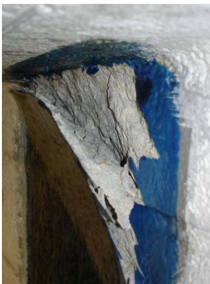
Figure 7.9 – B-2a Peeling of Laminate
